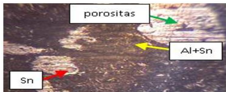
Figure 5. Microstructure of Al–Sn powder alloy composite (Al 60%–Sn 40%), 200× magnification
